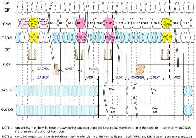
NOTE 2 CA to DQ mapping change via MR 48 omitted here for clarity of the timing diagram. Both MR41 and MR48 training sequences must be completed before exiting the training mode (MR42). To enable a CA to DQ mapping change, CKE must be driven HIGH prior to issuance of the MRW 48 command. For details, please refer to CA Training Sequence section.
