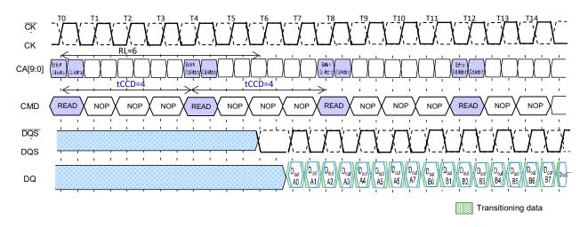
The seamless burst READ operation is supported by enabling a READ command at every fourth clock cycle for BL = 8 operation. This operation is supported as long as the banks are activated, whether the accesses read the same or different banks.
