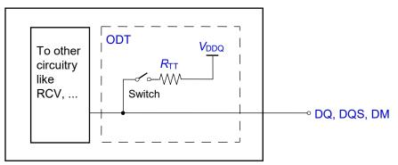
The switch is enabled by the internal ODT control logic, which uses the external ODT pin and other mode register control information. The value of *R*TT is determined by the settings of mode register bits.
