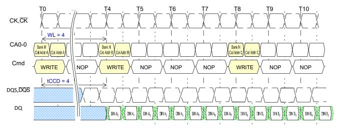
NOTE 1 The seamless burst WRITE operation is supported by enabling a write command every four clocks for BL = 8 operation. This operation is supported for any activated bank.
