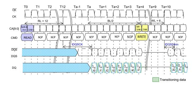
The minimum time from the burst READ command to the burst WRITE command is defined by the read latency (RL) and the burst length (BL). Minimum READ-to-WRITE latency is RL + RU(tDQSCK(MAX)/tCK) + BL/2 + 1 - WL clock cycles.
