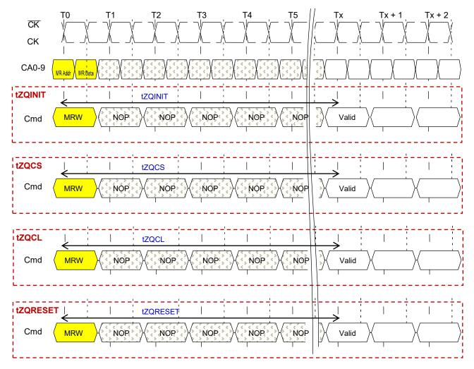
NOTE 1 Only the NOP command is supported during ZQ calibration.
