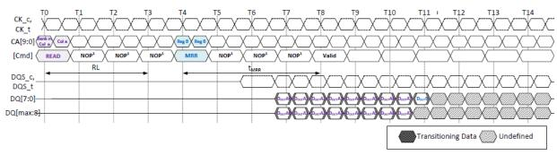
NOTE 1 The minimum number of clock cycles from the burst READ command to the MRR command is BL/2. NOTE 2 Only the NOP command is supported during tMRR.
