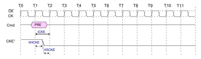
NOTE 1 CKE can go LOW tIHCKE after the clock on which the PRECHARGE command is registered.
