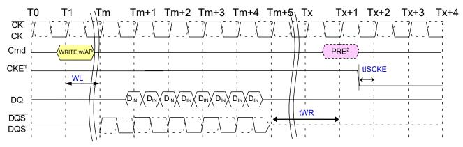
NOTE 1 CKE can be registered LOW at WL + 1 + BL/2 + RU(tWR/tCK) + 1 clock cycles after the WRITE command is registered. NOTE 2 Start internal PRECHARGE.
