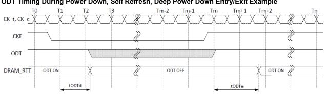
ODT Timing During Power Down, Self Refresh, Deep Power Down Entry/Exit Example
